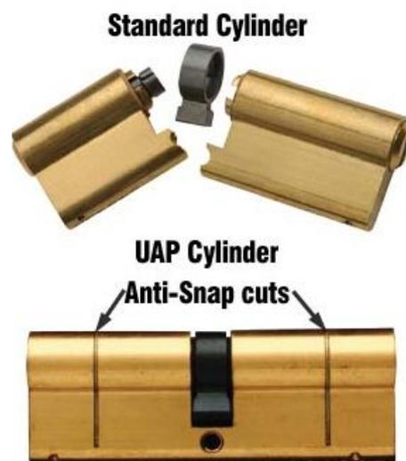
The thief first has to gain access to the cylinder. Once this has been done the cylinder can be easily snapped at the weakest point by force, giving the thief access to the lock cams which enables them to open the door.
